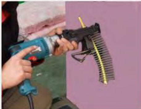
Screw gun with auto-feed belt
